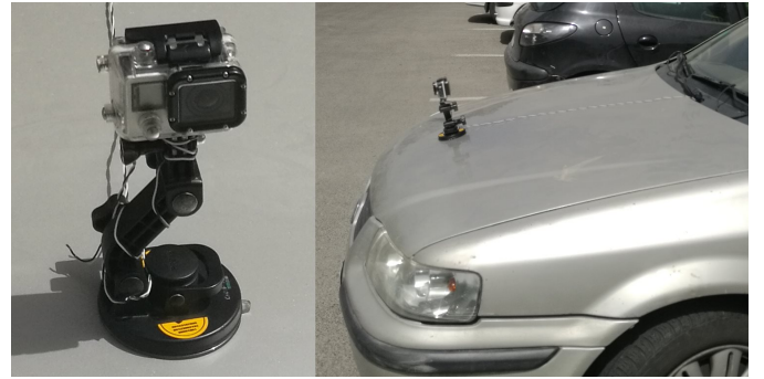
Fig. 2: GoPro camera is used in our experiment and attached to the hood of the car.
